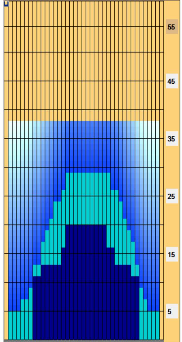
This pattern is for lane machines with a transfer brush and "drop brush" software. Older machines with a transfer roller can also use this pattern unaltered. If you are not sure or have a transfer brush machine without "drop brush" please contact Graeme Rose at [graeme@tenpintec.com.au](mailto:graeme@tenpintec.com.au).
